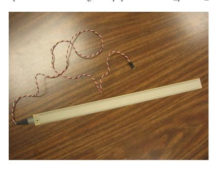
Force-sensitive Resistor (FSR)
