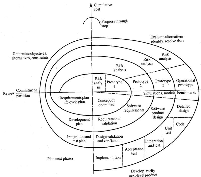
Picture 21: Spiral model of software process (Boehm, 1988)
