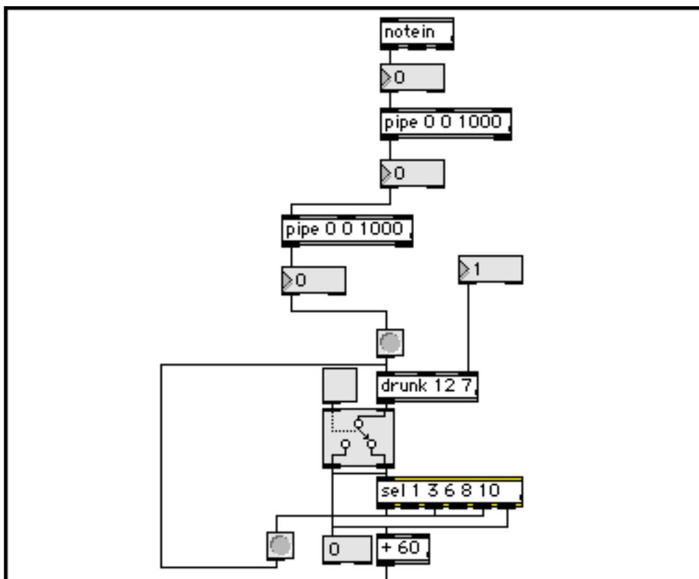
Figure 4-3: Max/MSP patch for the harmony generator engine.
